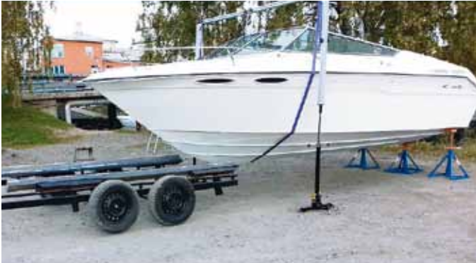
The stern placed on boat stands and the front lifted. The trailer picking up the boat after the keel stand, trestles or other bow support has been taking away.
